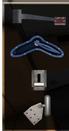
**UPPER DOOR HANDLE:** The upper handle will un-latch the upper section of the door. To un-latch the motor hook must be un-hooked. To latch the upper door handle, the motor hooks must be hooked. The motor hooks must be motored back to the un-hooked position after the door is latched otherwise the red DOOR annunciator will illuminate.
