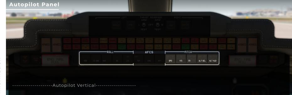
**SPD:** The SPD mode is used to maintain the airspeed or Mach at the moment of mode engagement by commanding pitch attitude changes.
